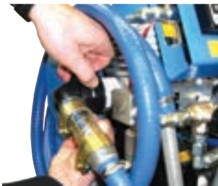
FA 016 with screwed-in suction strainer set FA 016.1775
